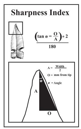
FIGURE 7.4. Calculation method for the sharpness index.
