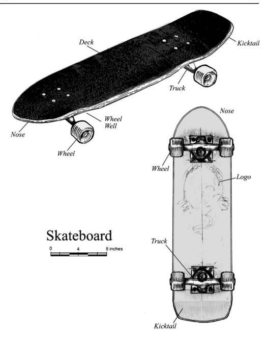
Fig. 2 Skateboard profiles with labels of parts
